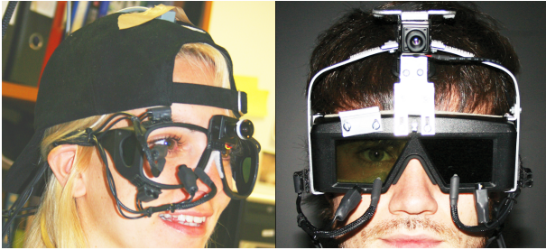
Figure 5. Eye tracker mounted on the WALL's lens-free frame (left), and on the ReaCToR's CrystalEyes® 3 shutter glasses (right).
