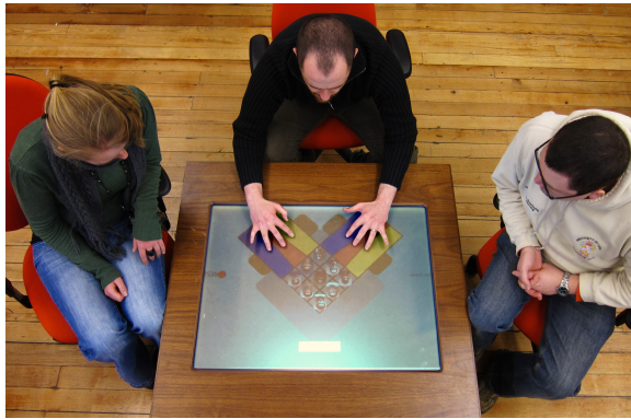
Figure 7. The FTIR table used for the evaluation 49 \times 95 \times 105\text{cm} , and the user study context.
