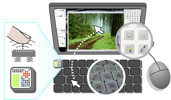
Figure 1. The Touch-Display Keyboard: each key is augmented with a touch-sensor and a graphics display. This enables interaction with graphical elements across keyboard and primary display device.
