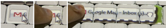
(a) Controls enter a resizing state when both mouse and finger are over the associated key, and the mouse can be dragged for resizing.
