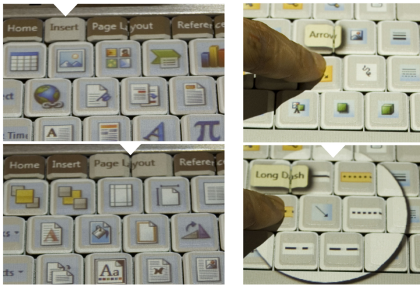
(a) Each function key acts as graphical tabulators, activating a different temporary overlay of adjacent keyboard interface (example from Microsoft Word). (b) Pie menus allow the temporary overloading of adjacent keys, eg. to provide refinement of a command.
