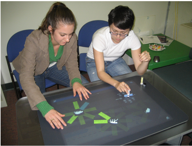
Figure 6. Interacting with BLAST results of the human TP53 gene against the mouse, rat, and monkey genomes. A physical BLAST tool (shaped as a spacecraft) presents a star-shaped search menu when placed upon the surface. Search results are organized in a flower-like structure around a target organism, with bright results represent high similarity score.
