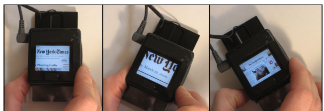
Figure 6. A user can pan around a document by translating the device. Zoom level is controlled by twisting clockwise or counterclockwise. After a motion is completed, the device can be lifted and reoriented (similar to mouse clutching).
