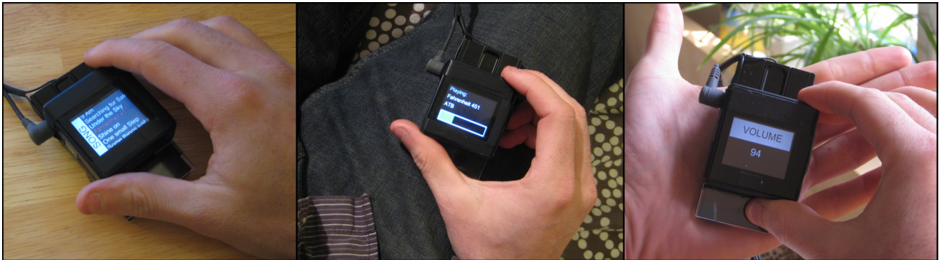
Figure 1. Our prototype Minput -augmented device running an audio player application. Two optical sensors on the back of the device enable x/y translation and rotational tracking on ad hoc surfaces, such as tables, walls, clothes, and the palm of one's hand.
