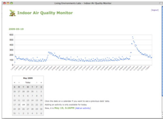
Figure 4. inAir website showing 24 hours of data of one of the participants. The two spikes in the graph correspond to 7am (breakfast) and 8pm (dinner) at the left/right respectively.
