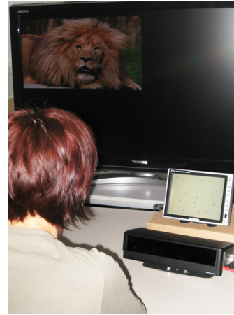
Figure 3. Setup of the fixation study. Participant performs a search task on an 8” display and his attention as grabbed by animal pictures on a 42”.
