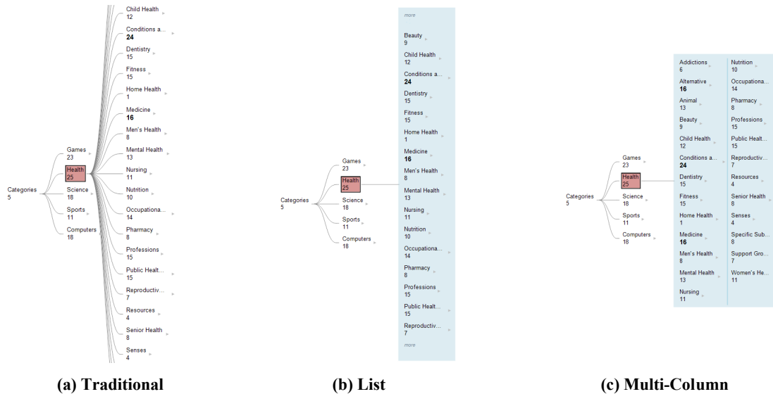
Figure 1. Three Tree Visualization Interfaces: Traditional (TRD), List (LST), and Multi-Column (MLC). TRD interface unfolds all child nodes in the traditional way. LST interface shows child nodes in a list with a cue node with the word, “more,” indicating that there are more invisible ones. MLC interface shows all children in a tabular display with multiple columns.
