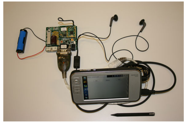
Figure 2. The components used for the SensorTune prototype: N800 PDA, TinyNode and headphones.
