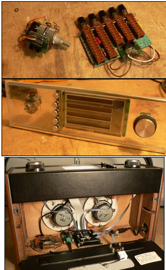
Figure 4. The digitally-enhanced original radio controls (top), the replacement control panel assembly (middle), and the assembled FM Radio (bottom)
