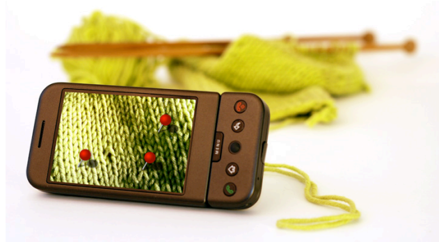
Figure 1. The current Spyn system runs on Android 1.5 G1 phones; vision recognition correlates recorded media with locations on fabric. Image courtesy of James Jordan.
