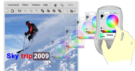
Figure 2 - LensMouse shows the floating color panel window of a drawing application. This reduces window management and minimizes on-screen occlusion.
