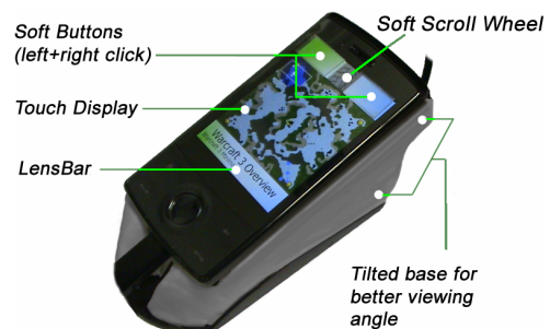
Figure 1 - LensMouse prototype showing an overview map from a real-time strategy game.
