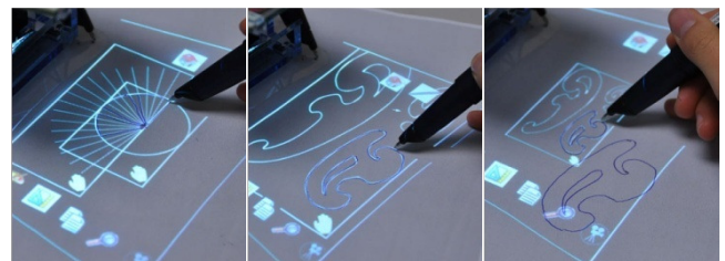
Figure 13 Drafting Tool feature. Left: Multiple draft and measuring tools can be used to guide drawing. Right: The viewport scroll wheel allows users to change the scale of the toolglass.
