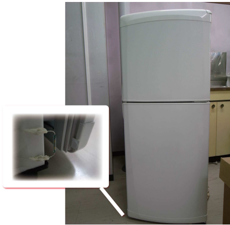
Figure 5. Sensor placement on refrigerator door – Lab B.
