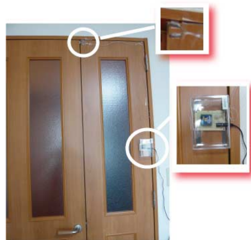
Figure 9. Sensor placement on door – House A.
