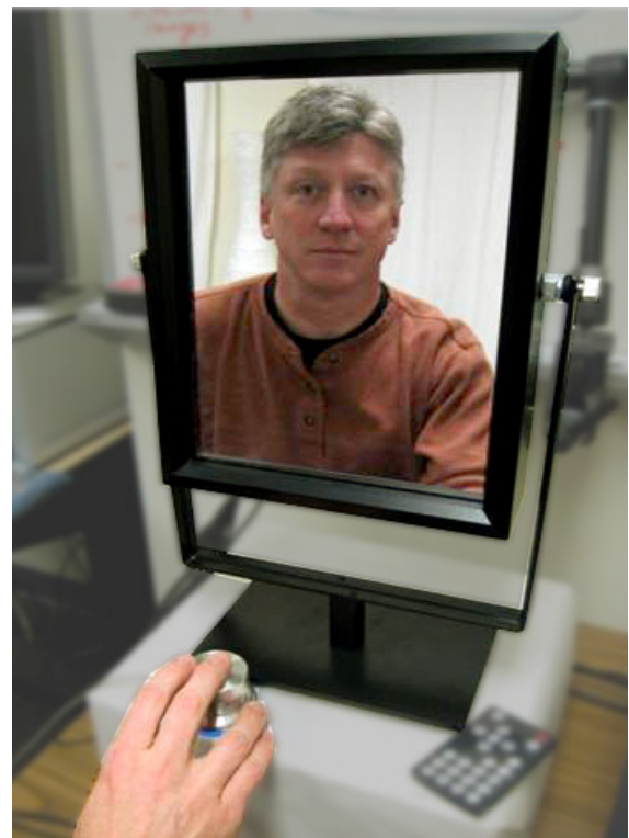
Figure 2. Countertop Responsive Mirror (P2). Mirror component consists of camera behind half-silvered mirror and a "record/stop recording" button..
