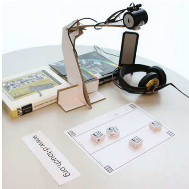
Figure 1: Setup of the d-touch system with the webcam, the active surface, the paper blocks and the speakers.
