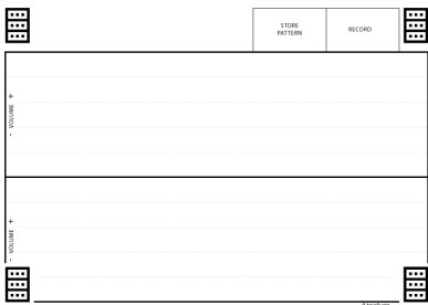
Figure 3: The d-touch sequencer. The x-position corresponds to the time instant within the loop, y-position relative to the track determines the playback volume. The two areas on the top right allow the recording of new sounds and to store the content of the playback area.
