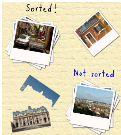
figure 5. Stacks of items formed via the Stapler pen+touch gesture. The user staples items by (1) tap-selecting a series of items, (2) holding a finger on the representative item for the stack, and then (3) tapping the pen on that item while continuing to hold it. The representative item appears on the top of the resulting stack.
