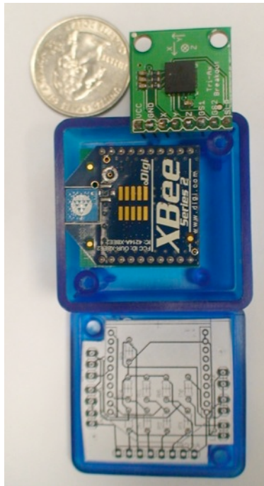
Figure 4: XBees accelerometer sensor box (with quarter shown for size comparison).
