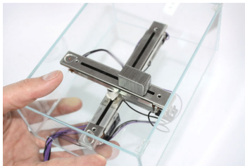
Fig. 2: Prototype. Weight-augmented box, containing an iron weight mounted to two motor faders.
