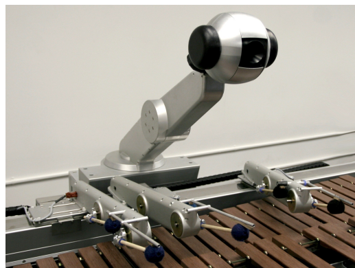
figure 2. The expressive head serves social communication. Shimon was designed in collaboration with Roberto Aimi of Alium Labs.
