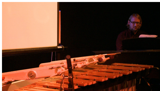
figure 3. Live human-robot Jazz performance using the system described in this paper (not including the social head).
