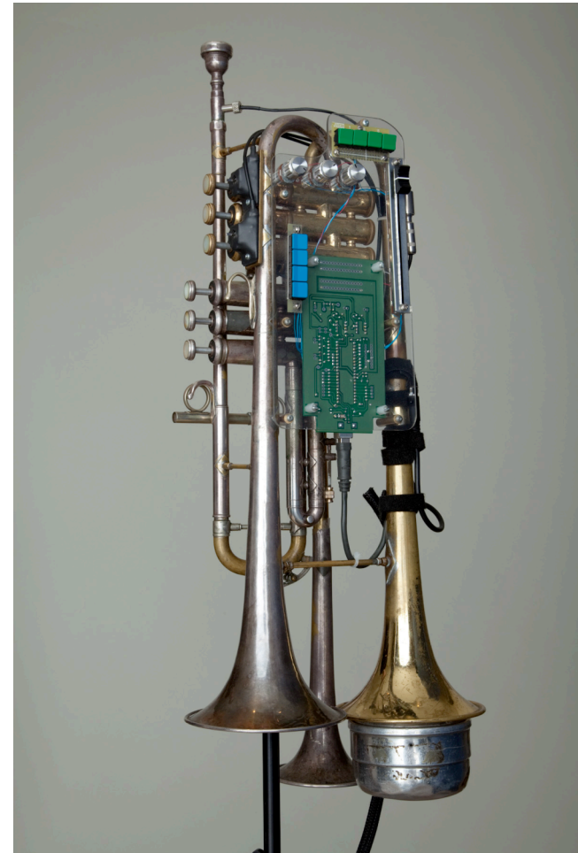
figure 1 – the mutantrumpet , designed by Ben Neill, with STEIM Junxion board and multiple MIDI controllers. Photograph by Eric Calvi
