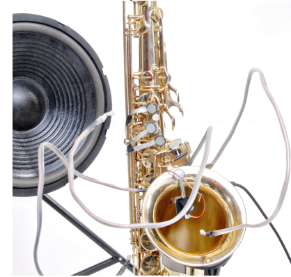
figure 2. The Metasaxophone microphone system
