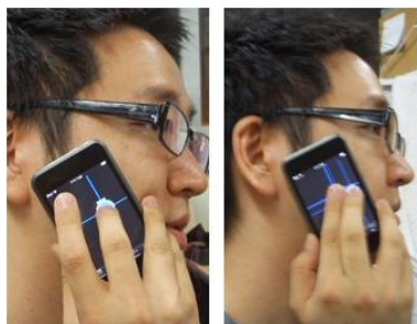
figure 2. Example of expressing touch behavior while speaking on the mobile phone using index and middle finger
