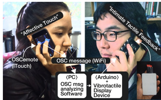
figure 3. Structure of CheekTouch prototype
