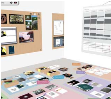
Figure 3. The CloudRoom consists of three planes with distinct functionalities. The left-hand wall holds work-in-progress, the floor is long-term, persistent storage, and the right-hand wall displays the timeline overview.
