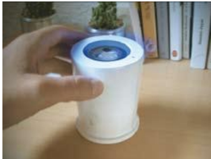
figure 3. Pot rotation for volume control.
