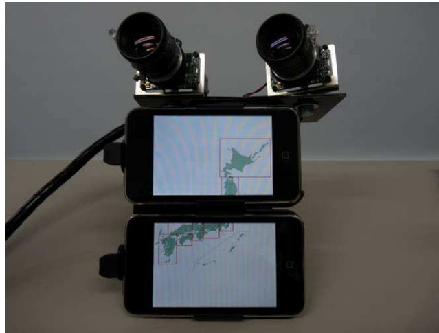
figure 8. Dual screen type: It is no longer possible to operate such a mobile device with one hand.
