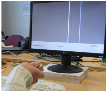
figure 5. Experimental task. The user performs reciprocal 1D pointing tasks by rotating the wrist while holding a small object. Rotations are detected by a magnetic system. Selections are activated by pushing a key on the keyboard with the non-dominant hand. Note that the hand is not externally constrained and movement is natural.
