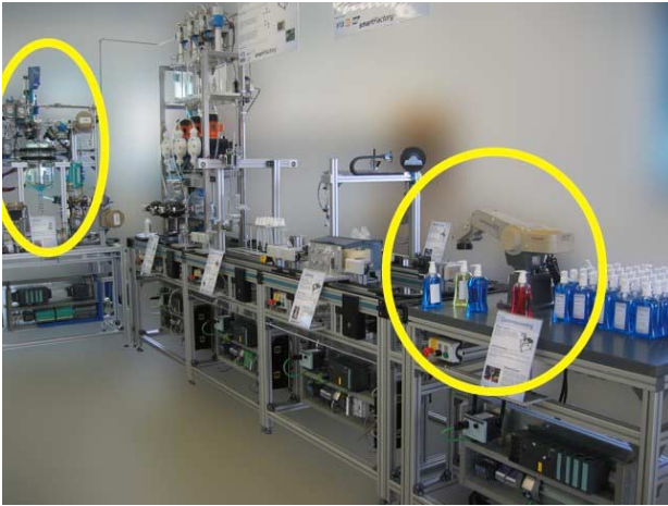
Figure 3: The production of personalized soap dispensers in the SmartFactoryKL . Color mixing unit (left) and personalized soap dispensers (right).
