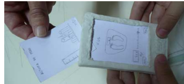
figure 6. Initial low-fidelity prototypes used during the early stage evaluation sessions. The designer is switching the various sketches/screens while the child uses the device.
