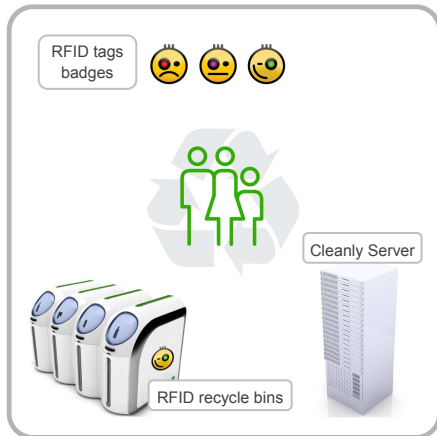
Figure 5: Cleanly artifacts including RFID bins, data server, and badges. Trashcan ID design by Woo S. Park.
