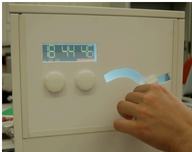
Figure 4: A first proof-of-concept toolkit to build an alarm clock with tangible user interface.
