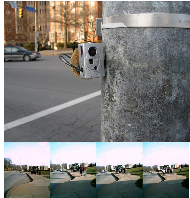
Figure 2: Top: A keychain camera is hacked via a microcontroller and outfitted with magnets for placement on a traffic pole near a bus stop. Bottom: Examples of time-lapse photographs retrieved from the keychain camera. Current camera resolution is 300 by 200 pixels from a $10 camera.
