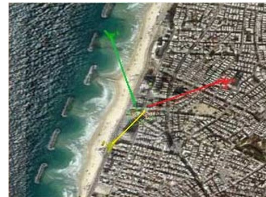
figure 1. UAV's on the command and control map. Here operators can view the location of all UAVs in the arena. Specifically in this example there are three UAVs (marked in red, green and yellow).
