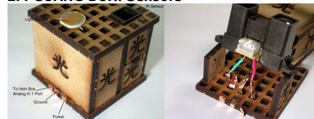
Figure 5: The GUANG BOX consists of a photocell sensor and an infrared ray sensor.
