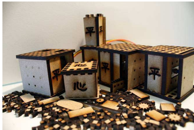
Figure 1. The TOPAOKO kit is made of laser cut hardboard embedded with circuit.
