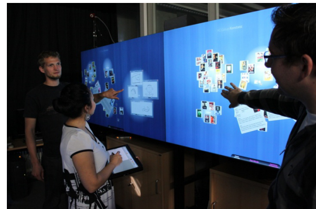
figure 3. Spatial positioning and scaling of artifacts on a zoomable pin board allows for different arrangements like timelines or process maps for cooperative reasoning. The visualization on an interactive whiteboard allows viewing, navigating, annotating and gesturing on artifacts.
