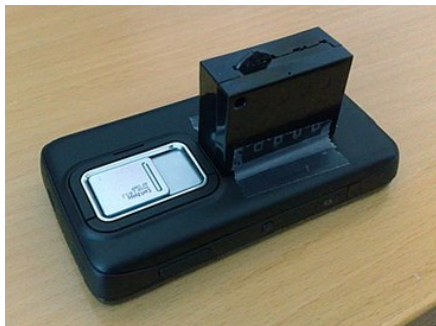
Figure 3. The hardware used for the MAA prototype: Nokia N900 with an external sensor module attached.
