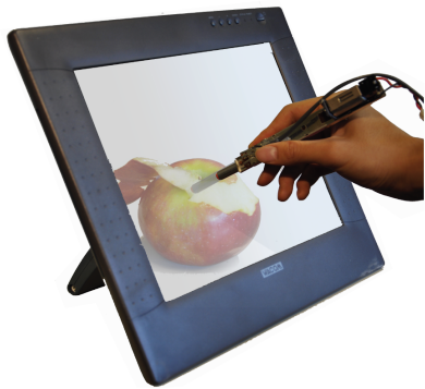
figure 6. A more portable version of Beyond prototype, using camera based tracking and a touch screen.
