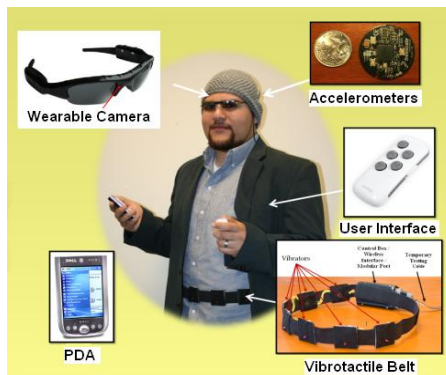
figure 1. The Social Interaction Assistant [4] consists of a pair of ordinary sunglasses with a discreetly embedded video camera (for image and video processing), earphones (for audio output), vibrotactile belt (for haptic output), accelerometers (for motion analysis) and a small, lightweight processing element that can be placed in a backpack.
