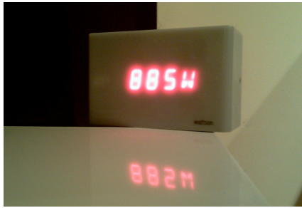
figure 1. The Wattson energy monitor from DIY Kyoto
