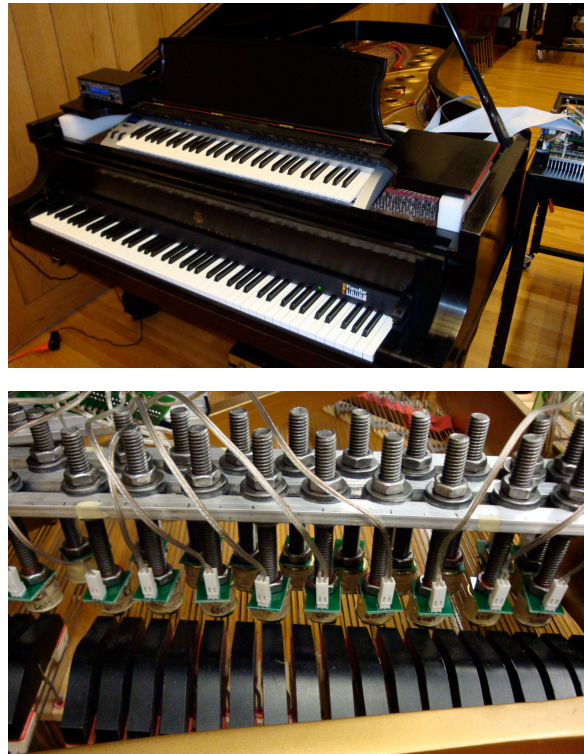
Figure 1: Keyboard sensor interface and electromagnetic actuators for an augmented grand piano.
