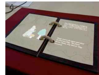
figure 3. Woody book covers, paper pages, and woody rings with magnets to bind pages and projected images onto pages.
