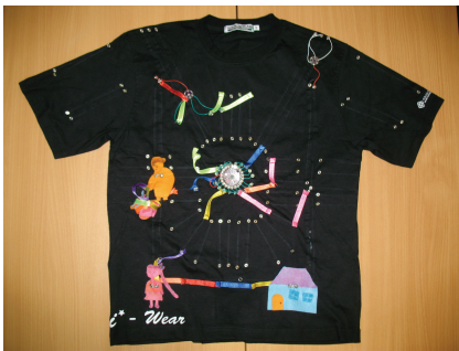
Figure 7. A project created by one of the TeeBoard/Lilypad workshop participants. Note the external connecting wires (encased in ribbons for insulation)
