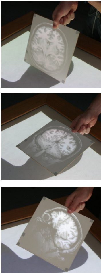
Figure 1. Users can slice through volumetric information spaces (e.g. an MRI scan of a human head) by arbitrarily moving or tilting the magic lens in the physical 3D space above a tabletop.
