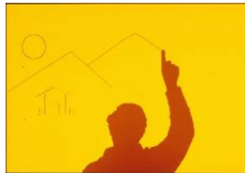
Figure 1. Here the index finger is recognized and when extended, becomes a drawing tool. Shaping the hand in a fist, so that the finger is no longer extended lets the hand be moved without inking [1]
