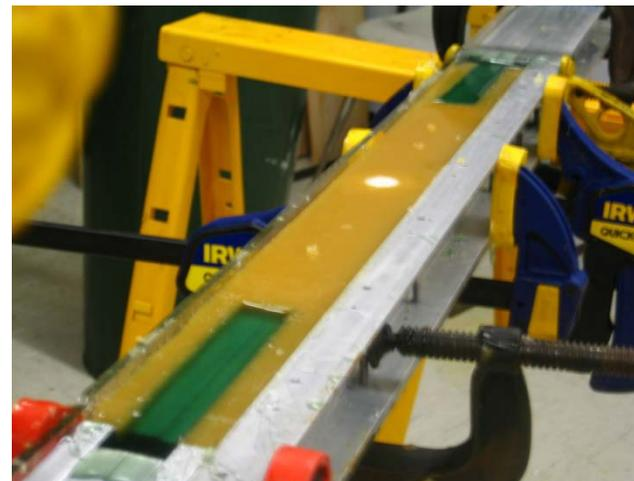
**figure 3.** The reconfigurable mold J (RCM-J) that fabricates all the parts that make up Open Columns
