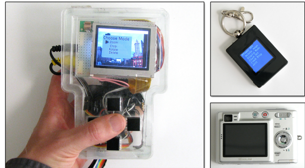
Figure 17. Participants were given a prototype device with a color display and button input. They were asked to revise designs for a keychain display and a digital camera, both running on the provided device.
