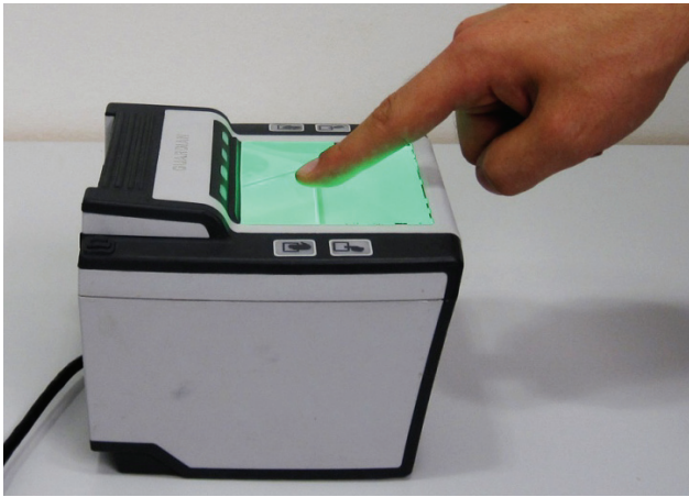
Figure 8: The RidgePad prototype is based on an L SCAN Guardian fingerprint scanner.
