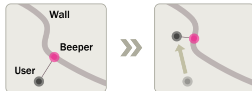
Figure 4. Beeper feedback. The beeper is placed along the wall, at the position with the shortest distance from the user.
