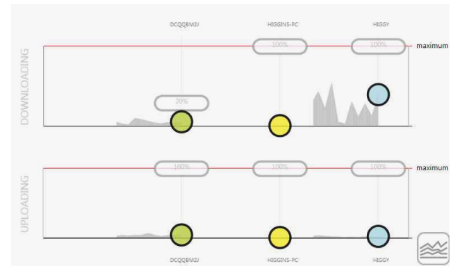
Figure 2: Current view showing real-time bandwidth usage for three home computers in Household D, including an applied download limit of 20% on the computer on the left.
