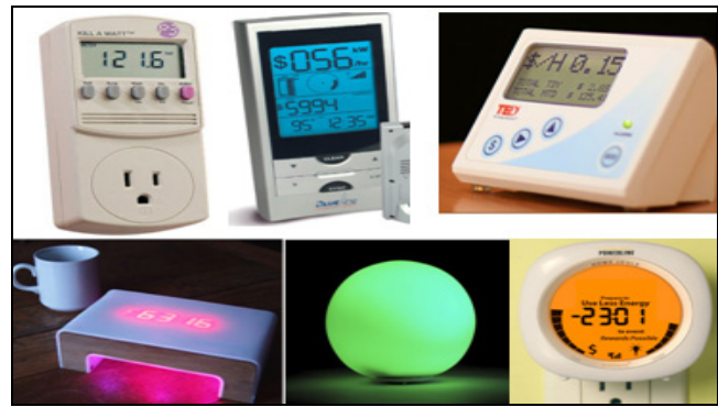
Figure 2. (Clockwise) Kill-A-Watt, Power Cost Monitor, Energy Detective, Energy Joule, Energy Orb, Wattson.
